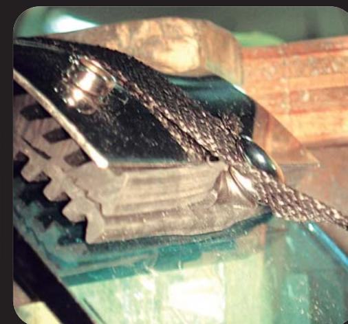
The M3 Canvas Clip exceeded a maximum load of 100 lbs. Canvas has an approx. strength of 80lbs/linear inch. Similarly, the strap that held the testing snap started to fray before a force greater than 100lbs. could be applied.
