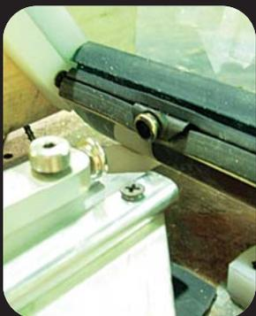
The M3 Canvas Clip was put through 10,000 cycles on a motorized tester (min. 13.5 years of use)...
